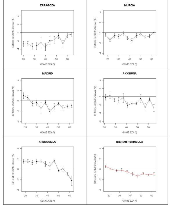
Figure 5: Variation of relative differences with the GOME solar zenith angle for cloud-free cases
